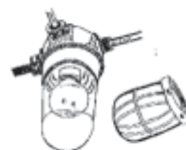
Figure 2. Light Fixture, dust and moisture-tight globe and wire cage to protect globe
