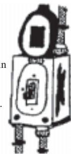
Figure 1. Switchbox. UF cable with dust and moisture-tight connections and cover
